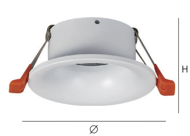
Model No: YZ5639 灯面尺寸 Lamp surface size: Ø90mm 开孔尺寸 Hole size: Ø68mm 灯体高度 Height of lamp body: 39mm
