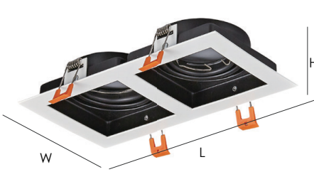
Model No: YZ5646 灯面尺寸 Lamp surface size: L220*W119mm 开孔尺寸 Hole size: Ø196*96mm 灯体高度 Height of lamp body: 37mm
