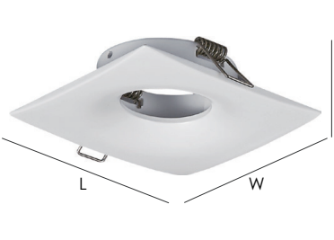
Model No: YZ5642 灯面尺寸 Lamp surface size: L98*W98mm 开孔尺寸 Hole size: Ø65mm 灯体高度 Height of lamp body: 27mm
