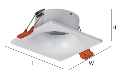
Model No: YZ5640 灯面尺寸 Lamp surface size: L91*W91mm 开孔尺寸 Hole size: Ø70mm 灯体高度 Height of lamp body: 30mm
