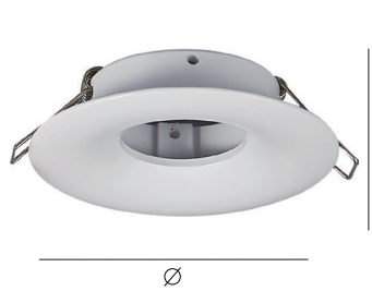
Model No: YZ5641 灯面尺寸 Lamp surface size: Ø98mm 开孔尺寸 Hole size: Ø65mm 灯体高度 Height of lamp body: 25mm
