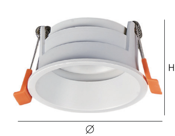
Model No: YZ5638 灯面尺寸 Lamp surface size: Ø78mm 开孔尺寸 Hole size: Ø68mm 灯体高度 Height of lamp body: 39mm
